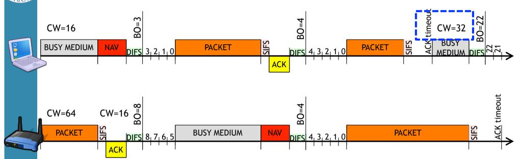
CW doubling after failure
